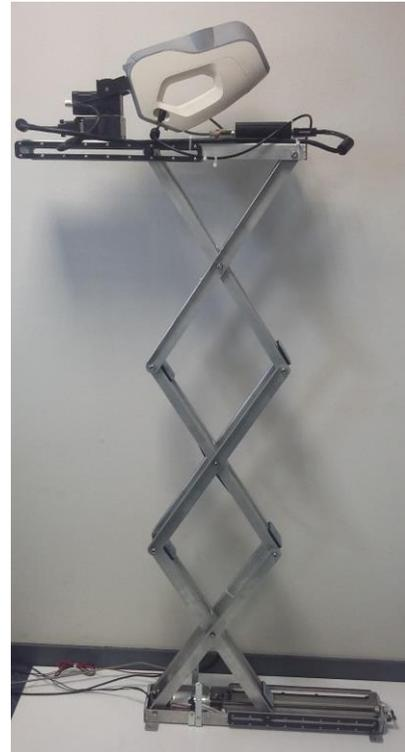
Fig. 11. Unfolded scanner positioning system.
